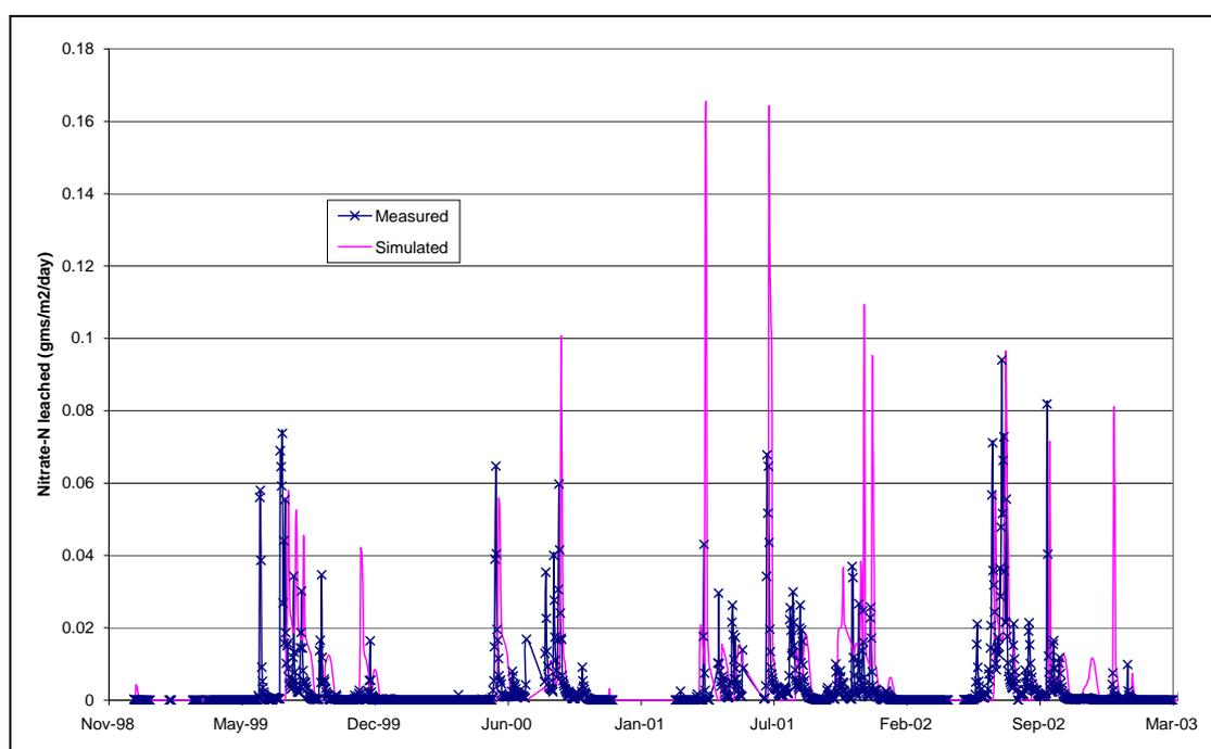
Figure 8: Simulated daily nitrate-N export ( $\text{g/m}^2/\text{day}$ ) compared to measured daily amounts from December 1998 through to May 2003 (note, only where measured data was available is the comparison made with the daily simulated data)
