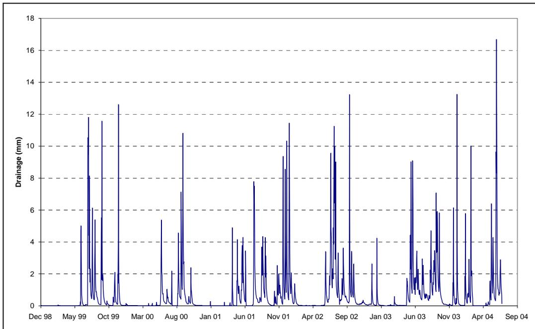
Figure 4: Measured artificial drainage flow from Toenepi from Dec 1998 to Jun 2004
