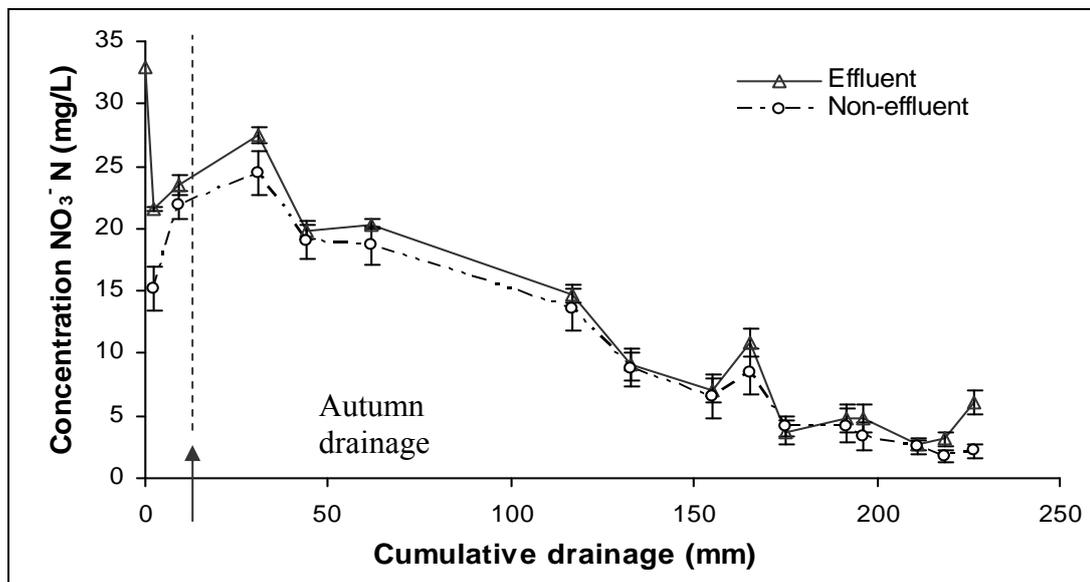
Figure 3: Trend in nitrate-N concentrations with accumulated drainage (Houlbrooke et al, 2003)
