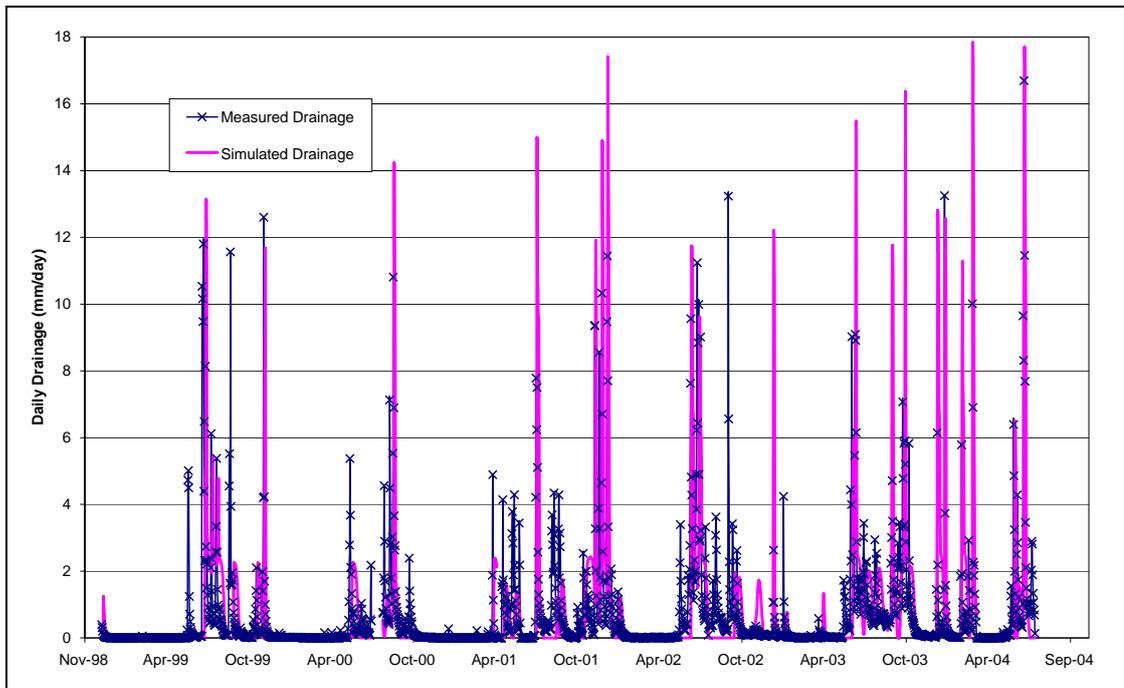
Figure 7: Simulated subsurface drainage compared to the measured data (on an event basis for the Howie artificial drainage system)
