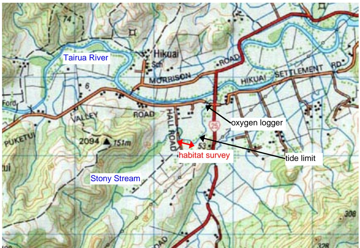
**Figure 2.3: Stony Stream.** Habitat was surveyed downstream of Hikuai Hall Rd (red arrow), and upstream of the measured tidal limit. Dissolved oxygen was monitored continuously at Puketui Valley Road. Tairua township is 10 km to the north-east.
