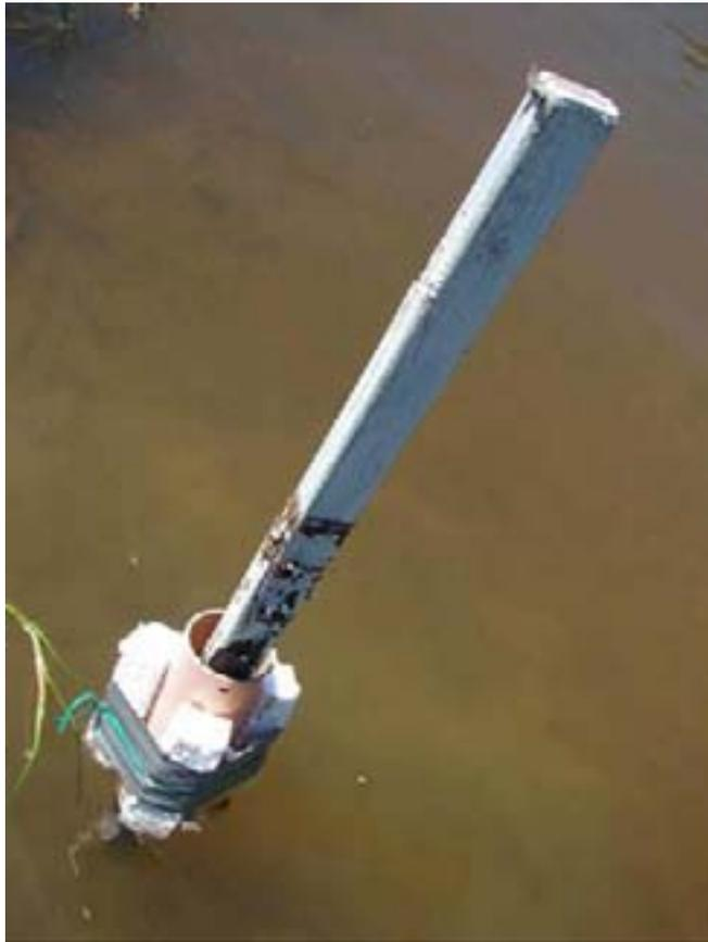
**Figure 2.12:** The change in water level between high and low tide was measured using bark shavings to leave a water mark on the stake at high tide. The PVC tube (with floats) stopped the shavings from washing away.
