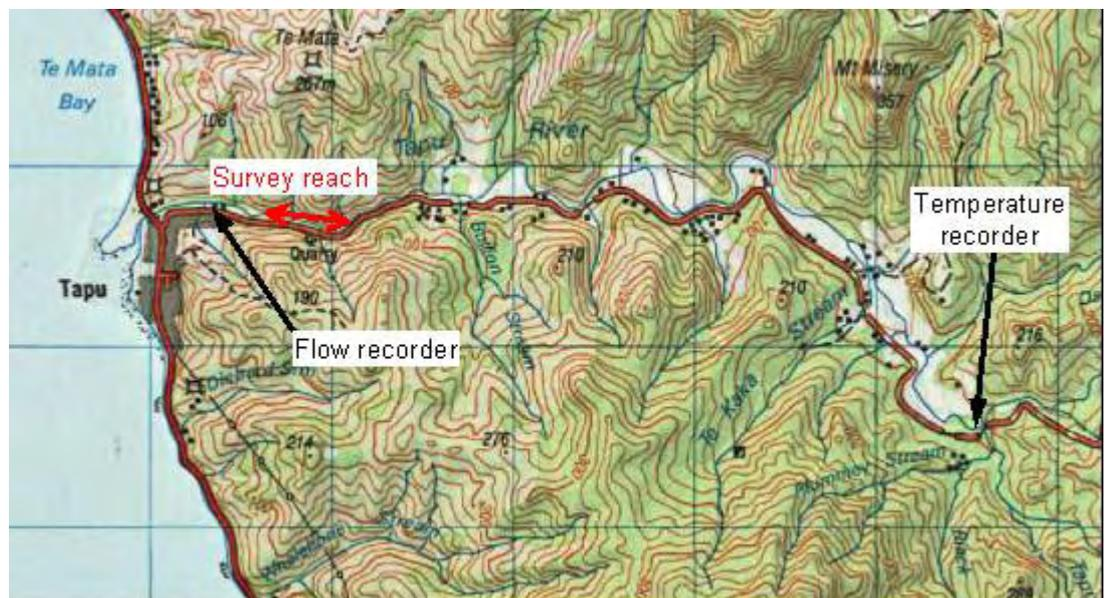
**Figure 2.6:** The survey reach on the Tapu River was a short distance upstream of Environment Waikato’s flow recorder. A temperature recorder was also installed several kilometres upstream. (See Appendix 2 for GPS coordinates).
