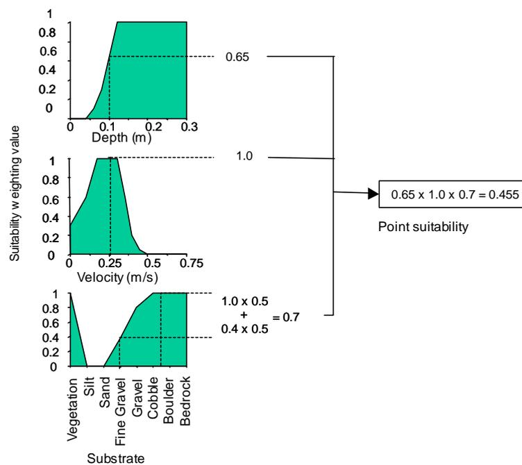
**Figure 1.8:** Calculation of habitat suitability for a fish species at a point with a depth of 0.1 m, velocity of 0.25 m/s, and substrate comprising 50% fine gravel and 50% cobble. The individual suitability weighting values for depth (0.65), velocity (1.0), and substrate (0.7) are multiplied together to give a combined point suitability of 0.455.
