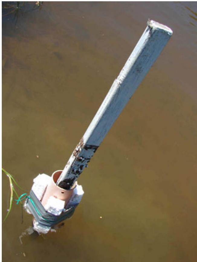
**Figure 2.6:** The change in water level between high and low tide was measured using bark shavings to leave a water mark on the stake at high tide. The PVC tube (with floats) stopped the shavings from washing away.
