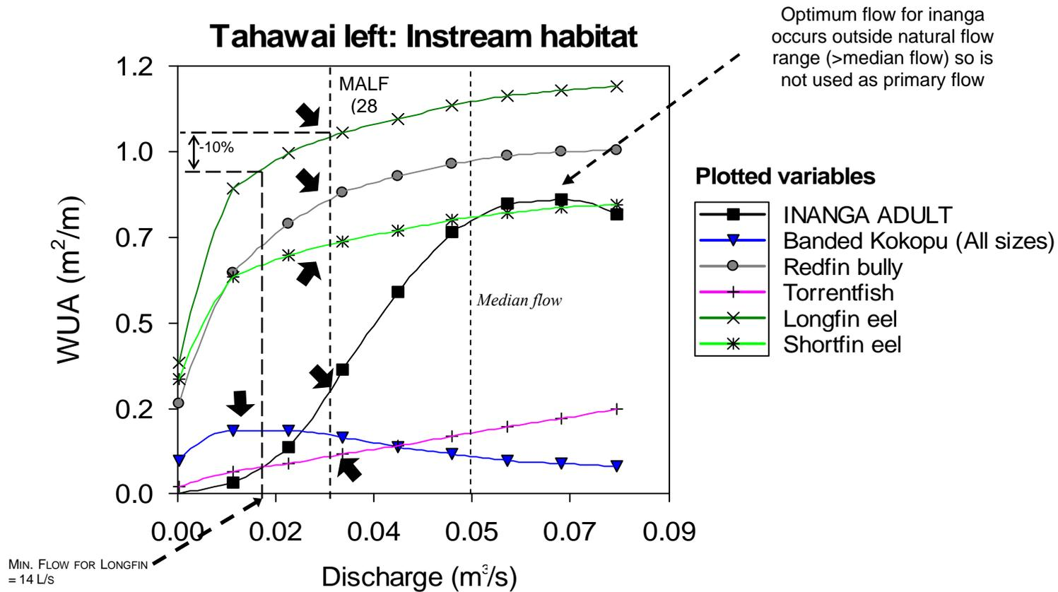
**Figure 1:** Modelled habitat for the Tahawai Stream (western BOP) expressed as habitat (WUA  $m^2/m$ ) versus flow. Primary flows determined using established criteria are arrowed for each species. Minimum flow calculation for longfin eel illustrated. Note, this is presented as an example only, as taxa and baseflow estimates were altered to illustrate the method.
