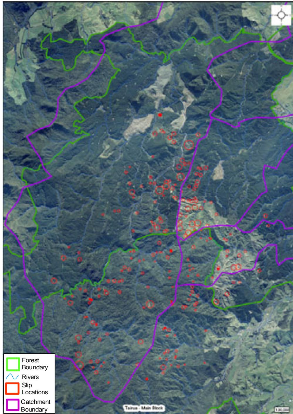
**Figure 3:** Aerial photo overlay of the central region of the Wharekawa River catchment (largest area enclosed by purple line) showing the proportion in pine forest (enclosed by green line) and the slips caused by the intense localised storm on 28 April 2006 (red circles). Figure provided by Kelvin Meredith of Rayonier.
