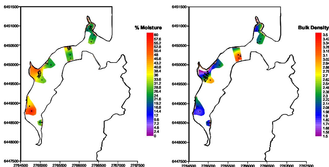
**Figure 8:** Spatial distribution of muddy sediments as indicated by high moisture content and low bulk density. High bulk density sediments correspond with firm sandy sediments. Sampling points used are plotted as dots.
