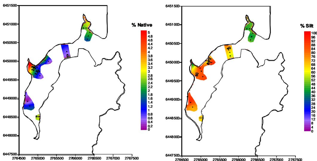
**Figure 14:** Plots showing the spatial distribution of soil contributions from native forest and ‘silt’ to the Wharekawa Estuary. The ‘silt’ includes bank erosion and fresh slip material. Sampling points used are plotted as dots.
