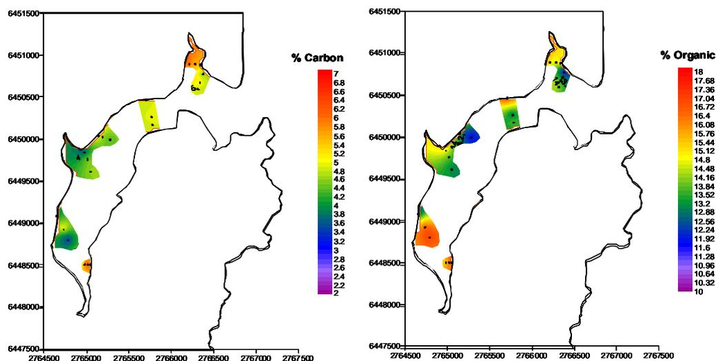
**Figure 9:** Spatial distribution of carbon and organic material in the bulk sediments. Highest organic content was associated with the sediment trapped in the mangroves. Sampling points used are plotted as dots.
