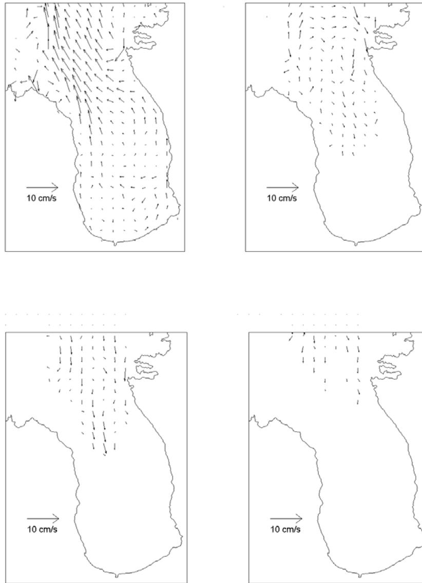
**Figure 15:** Simulated time-average currents during March 2000, using tides and temperature inputs, but no wind or river inflows. Plots are for horizontal layers, from upper right to lower left: 0-2 m, 8-10 m, 18-20 m, 28-30 m below mean sea level.
